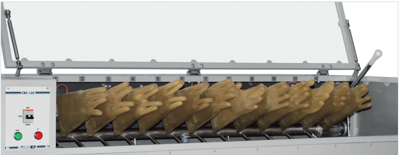
Testing dielectric gloves in CBC-12C bath
