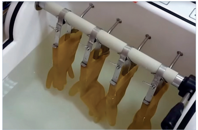
Testing dielectric gloves in CBC-C-series bath
