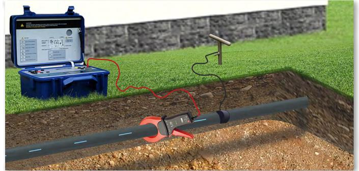
For this connection type you should close a clamp around the cable being located, which can typically be found near buildings or on utility poles; in some cases to apply the clamp you might have to dig around the cable.
