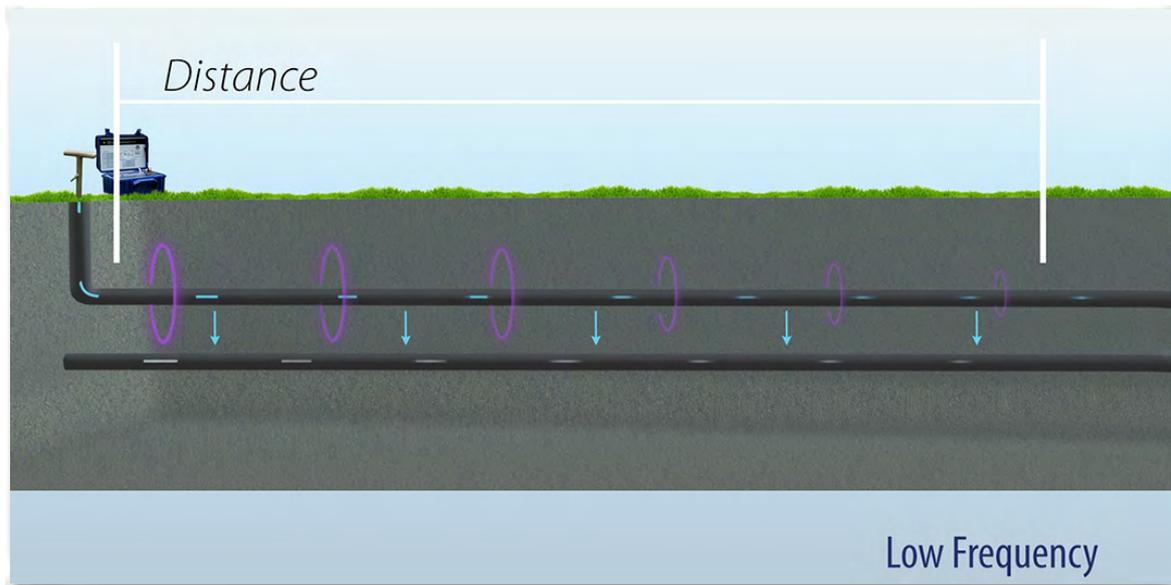
Therefore, in most cases it makes sense to start at the lowest possible frequency level and gradually increase the frequency as long as it is necessary.
