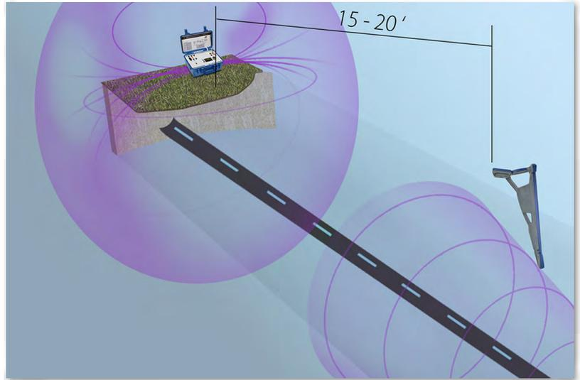
The problem with this method is that the signal it generates is considerably weaker than that produced in the conductive and inductive clamp methods. Also, nearby structures like cables located in the close proximity are likely to pick up the signal from the antenna and thus make the use of this method more difficult. This means that it is only sensible to resort to inductive locating if the other two active locating approaches cannot be applied.
