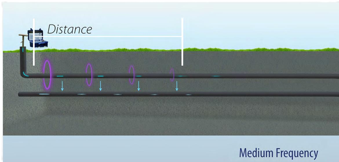
The choice of frequency depends on the locating conditions. In the best case scenario, with proper conductor connection and favourable soil conditions, it is a good idea to use the lowest frequency since the lower the frequency is, the farther the current will flow and the smaller the signal leakage to neighbouring objects will be.
