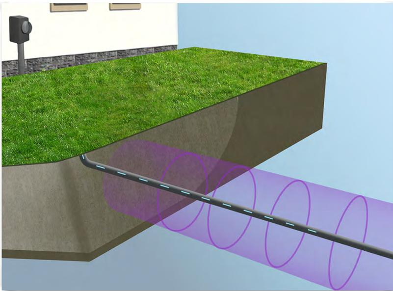
Passive cable locating is applied if the target cable is already electrically charged, in which case a transmitter is obviously not needed.
