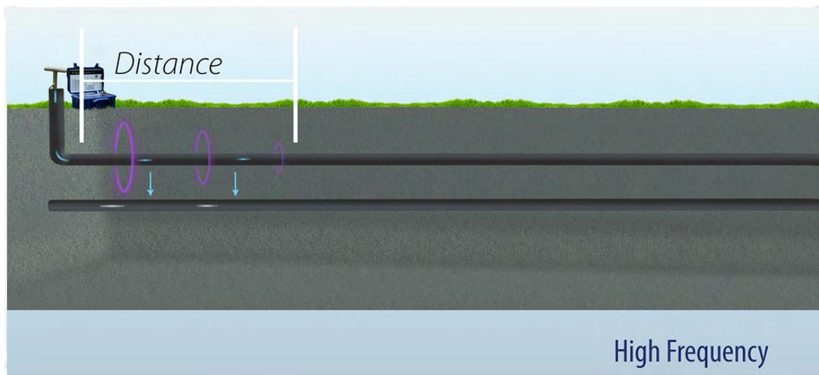
If you increase the frequency, the current will travel a smaller distance due to faster leaking, with a negative effect on the locating outcomes.
