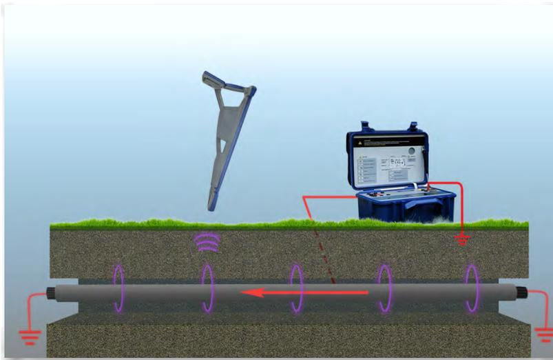
Active cable locating involves charging the target cable with electricity and then using a receiver to pick up the generated signal. For this type of location an electrical circuit, which will enable current to flow, is created according to one of three connection methods: conductive (direct), inductive clamp or inductive.
