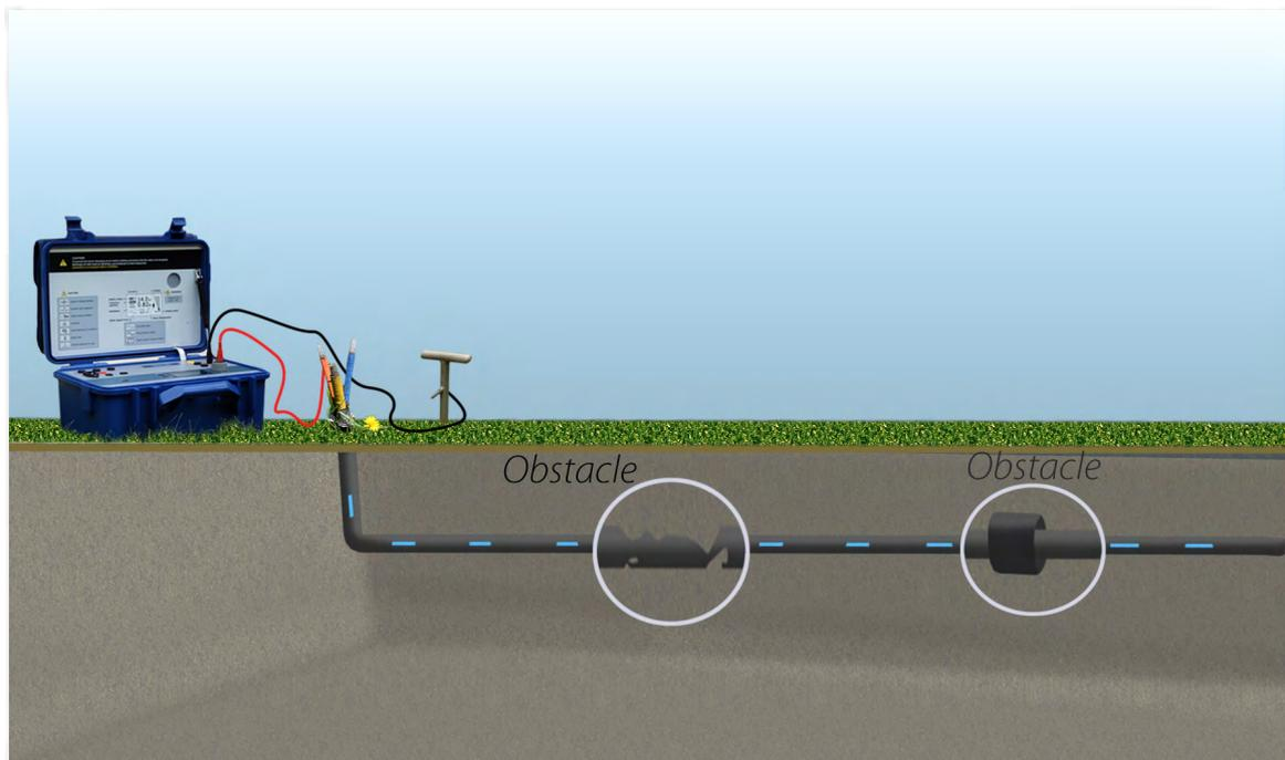
If locating conditions are not so good, with poor conductor connection, non-conductive elements, corrosion and other obstacles to the current flow, you will have to use a higher frequency to overcome these barriers.
