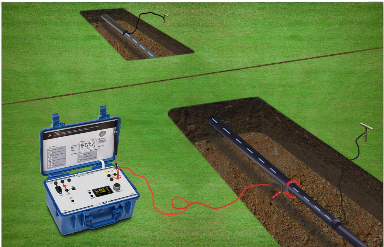
Fully close the clamp around the conductor at least on one end, but applying the clamp on both ends would make for better locating results. The line should also be earthed on both ends, otherwise the signal will be too low for cable locating. In case only one end of the cable can be earthed, it should be the far section of the cable. If not, the signal will travel to the near earthed end in a short time.
